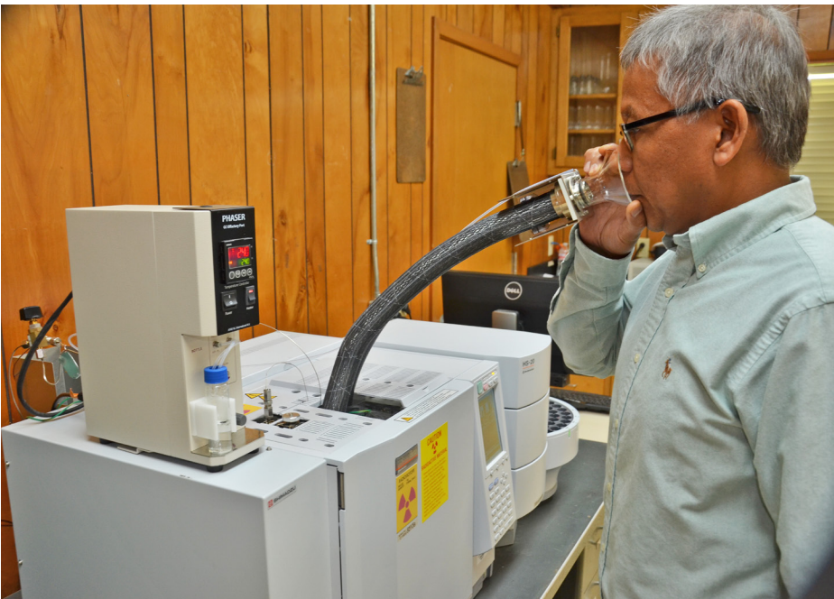
Manoch Kongchum, LSU AgCenter agronomy researcher, uses a gas chromatograph to detect both quantitatively and qualitatively the aroma found in Jasmine-type rice. The equipment was purchased with Louisiana Rice Research Board funds, and it also is being used to analyze air samples in a study of greenhouse gas emissions from rice fields.
